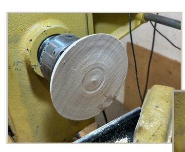
Mount lid on 4 jaw chuck and hollow out leaving a lip and couple of flat spots
