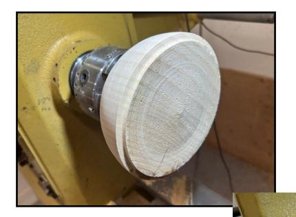
Mount bowl base on lathe using 4 jaw chuck and then turn tenon using lid as a fit check. Make sure lid fits snug but can still be taken off.
