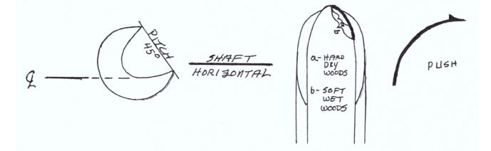
**FINISHING CUT** – Final cut on interior surface of open bowls in preparation for sanding.
